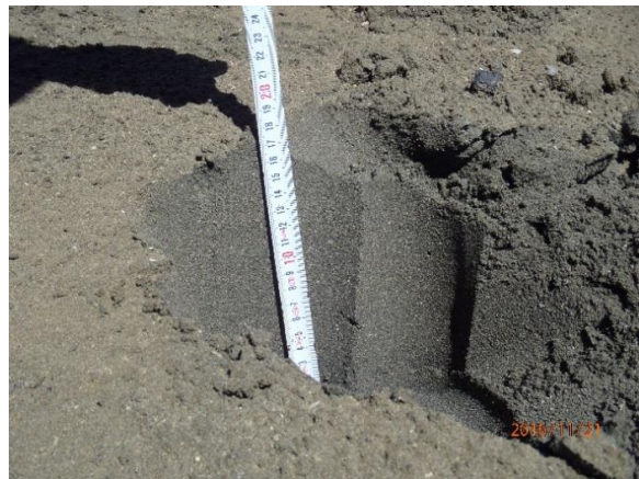
Figure 5.19: Sandy liquefaction ejecta with trace gravel among area of 1970's end-dumped quarry rock reclamation (i.e., Thorndon Reclamation) at STA 145 and approximately 60 m upland of the bulkhead. The ejecta deposit was approximately 170 mm thick at this location. Samples S11 and S12 were collected here (S41.279067°, E174.788792°, taken on 17NOV2016 and 21NOV16).
