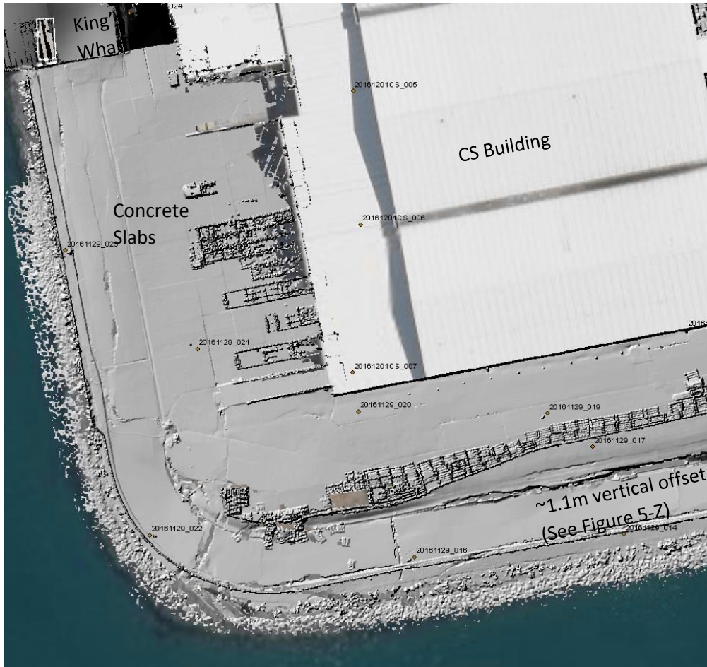
Figure 5.30: Example hillshade for the SW corner of the port, south of the CS building. This dataset was coarsely cleaned and still contains several artifacts from railing and metal racks.
