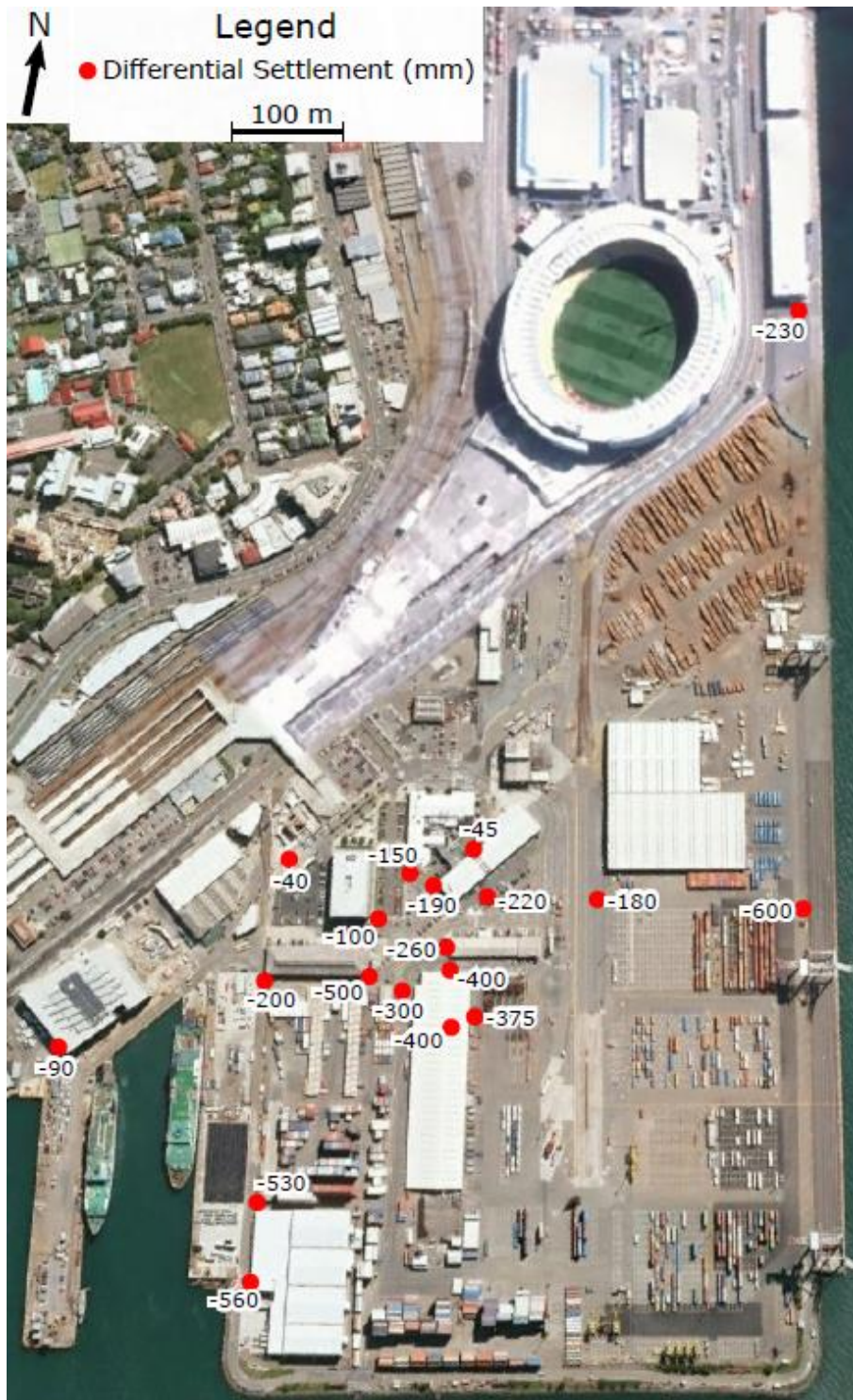
Figure 5.24: Location and magnitude of differential settlement measurements obtained during inspections. All values are in mm, and represent settlement of the ground surface relative to a pile supported structure. (Base image from Google Earth™)
