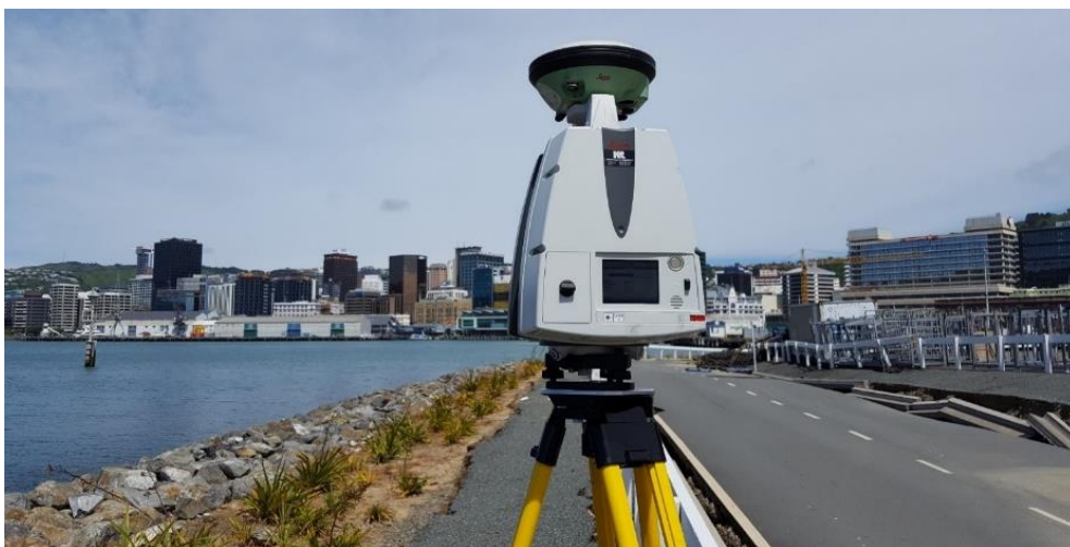
Figure 5.26: Example scan setup with a Leica P40 terrestrial laser scanner and Leica GS14 GNSS receiver mounted directly above the scanner.
