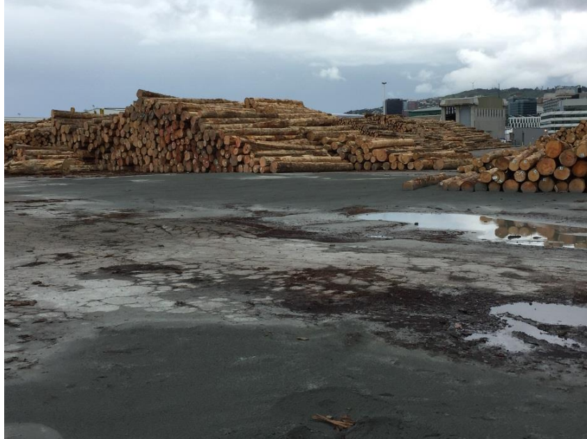
Figure 5.21: Sandy liquefaction ejecta in the log stacking area in the northeast corner of CentrePort (Sample S13). Area of hydraulic fill reclamation. (S41.274972°, E174.788347°, taken on 17 NOV16)
