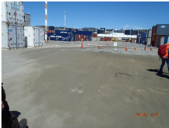
Figure 5.19: Sandy liquefaction ejecta with trace gravel among area of 1970's end-dumped quarry rock reclamation (i.e., Thorndon Reclamation) at STA 145 and approximately 60 m upland of the bulkhead. The ejecta deposit was approximately 170 mm thick at this location. Samples S11 and S12 were collected here (S41.279067°, E174.788792°, taken on 17NOV2016 and 21NOV16).
